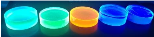
Fabricated 3" diameter plastic scintillators
